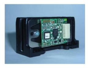
MSR170HK 43 mm USB HID Magnetic Stripe Swipe Card Read" consists of a high-performance multi-channel fully integrated magnetic stripe decoder chip at a low-profile magnetic read-head. This innovative, yet low-cost card reading solution offers many important advantages over the conventional less-integrated approach.
