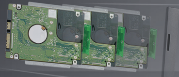
Equipped with 2.5" SATA drive slot and onboard M.2 SSD storage (option)
