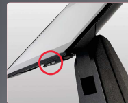
Power On/Off button & Status LED indicator for 13inch monitor
